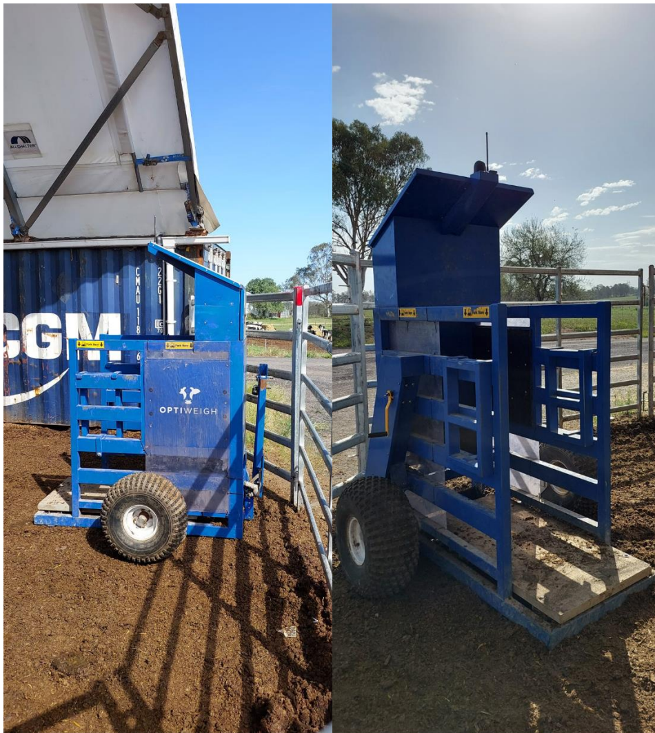
Figure 4. Agscent/Optiweigh utilized for measuring \text{CH}_4 and \text{CO}_2 emissions from individual animals.
